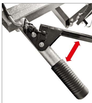
Fig.: Bowden cable on locking brake handle, right
