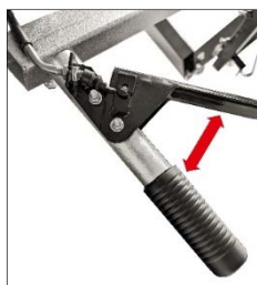
Fig.: Bowden cable on locking brake handle
