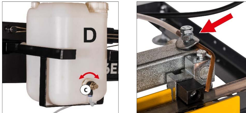
Fig.: Cooling the bandsaw blade
