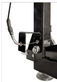
Fig.: Locking brake on chassis, right
