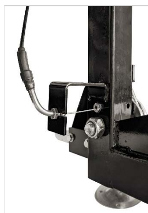
Fig.: Locking brake on chassis, right
